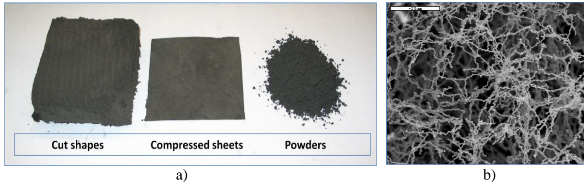
Figure 1: a) Nanostrand as-manufactured “cake” can be cut into shapes, pressed into sheets, or reduced to a nanostructured powder, b) SEM of nickel nanostrands, 1000 X (20 μm scale bar).
