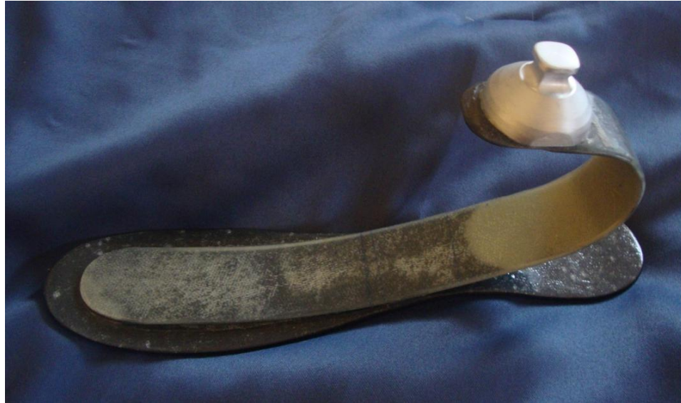
Figure 11: Prosthetic foot with nanostrand-polymer strain sensor integrated directly into the structure.
